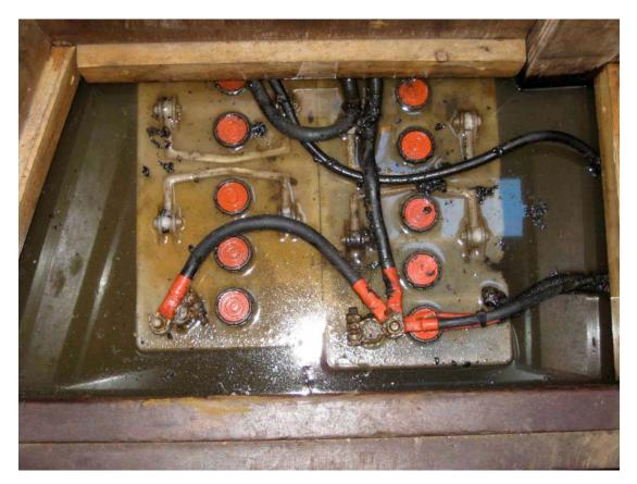
There were three domestic batteries and one engine battery onboard The batteries are charged by means of twin alternators.
